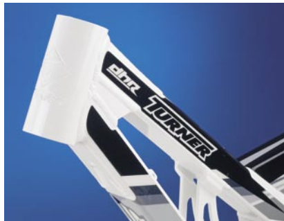
CNC-machined 1.5-inch head tube with top- and down-tube gussets
