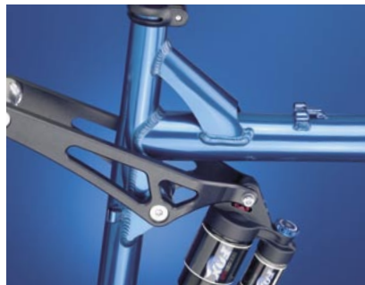
Light, strong CNC'd 6061 T-6 aluminum rocker arms (Fox DHX 5.0 Air shock standard; DHX 5.0 coil optional)
