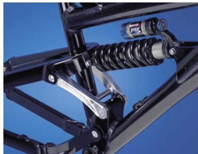
Fox DHX 5.0 coil spring shock with piggyback reservoir
