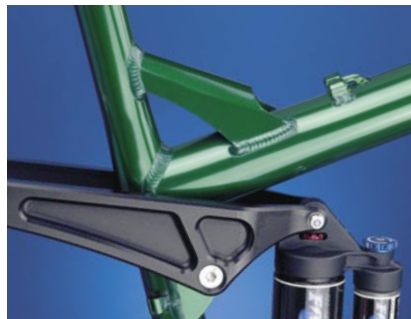
Sloping top tube with reinforced seat mast
