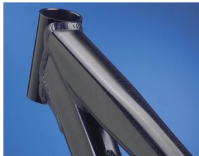
Custom-formed 6061 T-6 tubing, made in USA by Worth Aluminum
