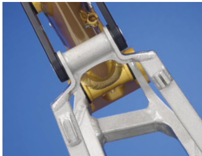
Super lightweight seatstay yoke and box section tubing. Maximum rider weight limit: 165 pounds
