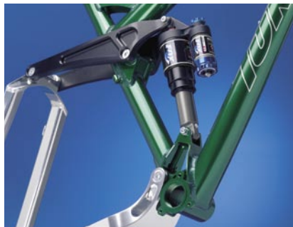
CNC-machined BB/swingarm pivot and chainstay yoke. (Fox DHX 5.0 coil shock standard; DHX 5.0 Air optional)
