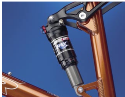
Fox's RP3 Air shock with lockout and adjustable compression/rebound damping comes standard
