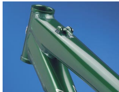
Butted and custom-formed 6061 T-6 aluminum tubing
